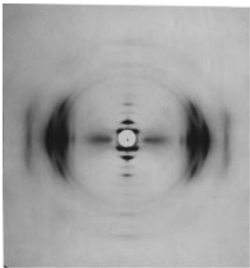
Figure 1. X-ray diffraction patterns for an oriented fiber of TQT-10H drawn from the nematic melt and annealed at 130 °C. The fiber axis is vertical.
